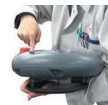
The teaching box can be held with one gripper by gripping the grip handle, and the enable switch operated with a finger on the same gripper. The other gripper can be used to operate the touch panel and buttons. The right and left grippers may be interchanged.
