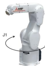
The J1 axis range of movement is limited by mechanical stoppers on the robot body and by the controller parameters. Use this feature when the range of movement needs to be limited due to problems such as interference with nearby devices.
