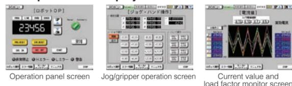
Enables the robot to be controlled from the GOT even without a teaching box. Current robot position data, error information, etc. can be displayed easily on the GOT.
