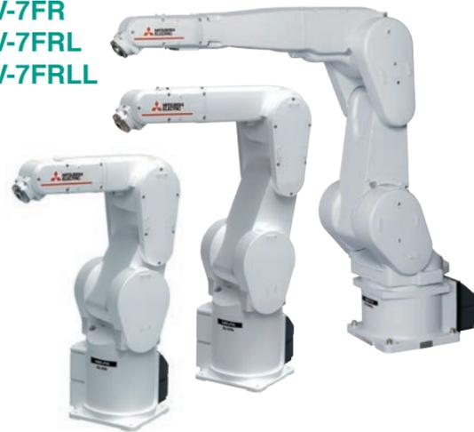
Cutting-edge servo control and optimized arm construction provide extremely fast and precise heavy-duty operation. Responds to Z-axis nudge requests. Increased range of movement along each axis and slender arms to cover large work areas. An ideal robot for compact cell construction. The product line includes a model with a maximum reach radius of 1503 mm for a larger operating range.
